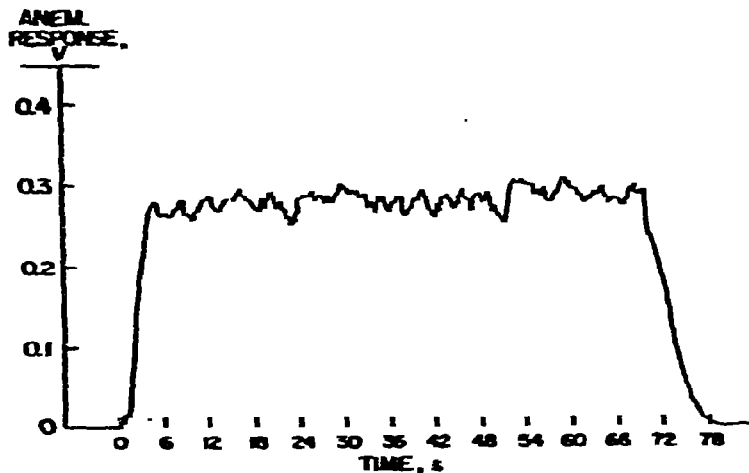
Fig. 4. Response for methane burning at a constant fuel feed rate.
